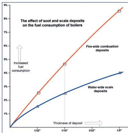
The adhesive properties of unburnt carbon result in a build-up of incombustible solids, ash, and carbon on heat transfer surfaces. The carbon and other deposits act as a thermal barrier, reducing heat transfer and boiler efficiency, and leading to higher stack temperatures in the boiler or air heater. The reduction in heat conductivity relates to a reduction in efficiency, as shown in the graph.
